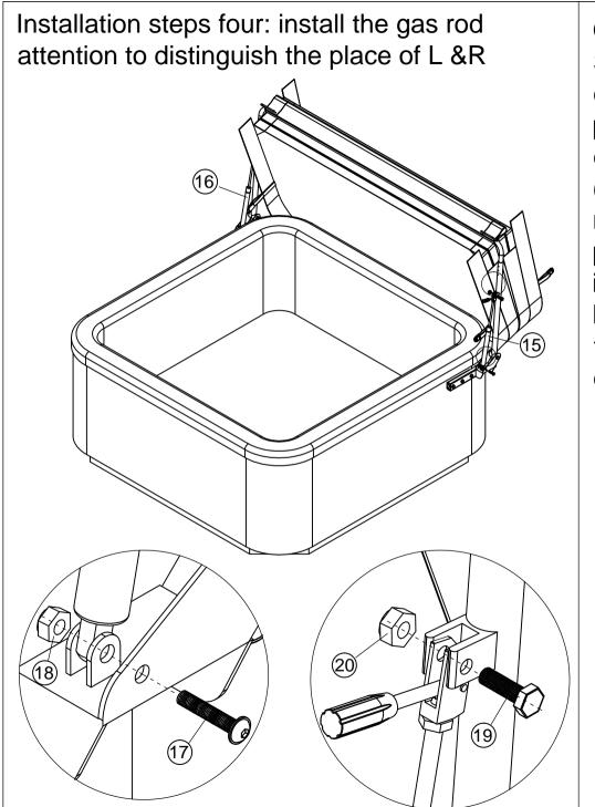
Operation method: this cover lifter with Self-locking positioning function. Each time to operating the spa cover open or closed, must press the operating lever counterclockwise, otherwise can't open or closed the spa cover. (operate as steps 1-2). When the operator releases the operating lever, the cover will position at the angle at which the current lock is opened.
