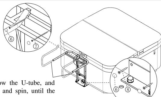
Press the protruding dots below the U-tube, and push the U-tube into the hole and spin, until the protruding dots in place and pop up.
