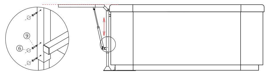
Inserted the product into the spa bottom, adjust the tipping frame up and down to let the highest position to be unanimous with the one of spa, and locking with the screws.
