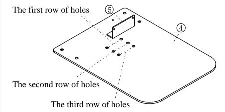
After installation, the distance from first row of holes to the skirt is 25MM, the second row of holes is 50 MM, and the third one is 75MM. Choose the closest size of your spa to install.
